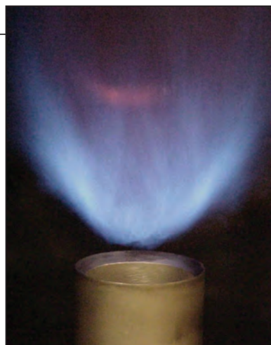
FIGURE 3. The interaction of the flows at the exit of the swirler assembly creates a flow profile that expands radially outward
