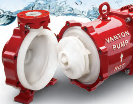
All wet end components of Vanton centrifugal pumps are molded of solid PVC, PP or PVDF, and handle flows to 1450 gpm (330 m 3 /h), heads to 400 ft (122 m) and temperatures to 275°F (135°C).
