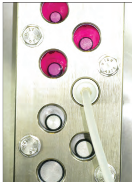
FIGURE 2. A reactant is being added to the fourth stage of a 10-stage Coflore ACR reactor
